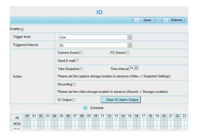
There is an IO alarm input / output lines in the FOSCAM camera tails. Enable IO alarm need this cable to connect to the alarm device (door sensor, infrared sensor, smoke detector, etc.).
