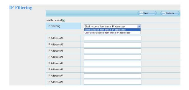
Enable firewall, If you select Only allow access from these IP addresses and fill in 8 IP addresses at most, only those clients whose IP addresses listed in the Only allow access from these IP addresses can access the Network Camera. If you select Block access from these IP addresses, only those clients whose IP addresses are in the IP list cannot access the Network Camera.
