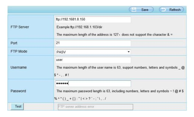
**FTP server**: If your FTP server is located on the LAN, you can set as Figure as above. If you have an FTP server which you can access on the internet, you can set as below.
