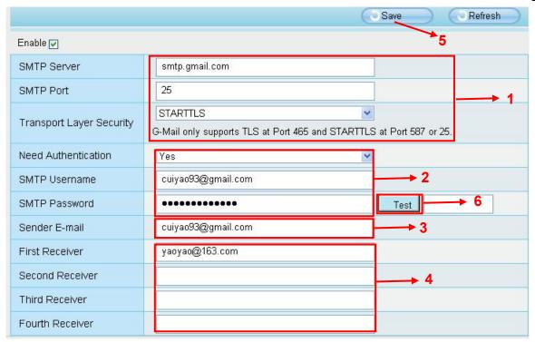
1----- SMTP Server / Port / Transport Layer Security Enter SMTP server for sender. SMTP port is usually set as 25. Some SMTP servers have their own port, such as 587 or 465, and Transport Layer Security usually is None. If you use Gmail, Transport Layer Security must be set to TLS or STARTTLS and SMTP Port must be set to 465 or 25 or 587, which port you choose should be decided by which Transport Layer Security you select.
