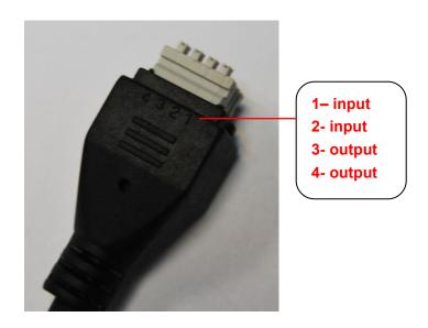
This camera supports I/O alarm, you can go to Settings-Alarm - I/O page to configure it.
