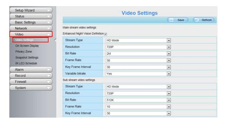
**Enhanced Night video Definition**: The camera will automatically drop the frame to extend the recording time in the night.
