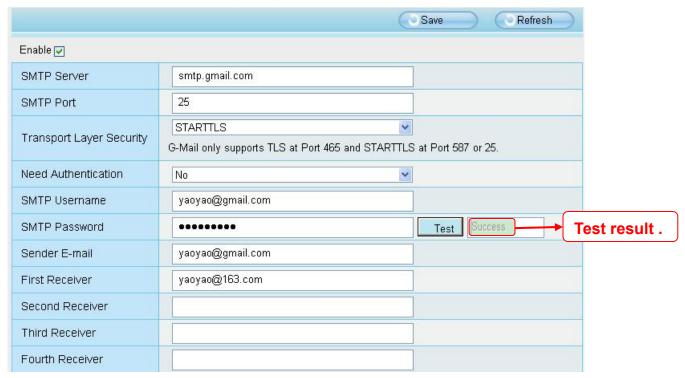
If the test success, you can see the Success behind the Test, at the same time the receivers will receive a test mail.
