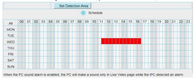
**7 Click Save** button to take effect. When the motion is detected during the detection time in the detection area, the camera will alarm and adopt the corresponding alarm indicators.
